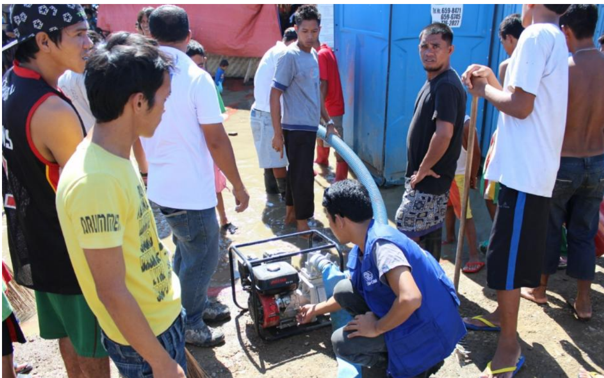
Gasoline-fuelled water pumps provided by ICRC/PRC and IOM were used to extract the flooding in Zone C.
